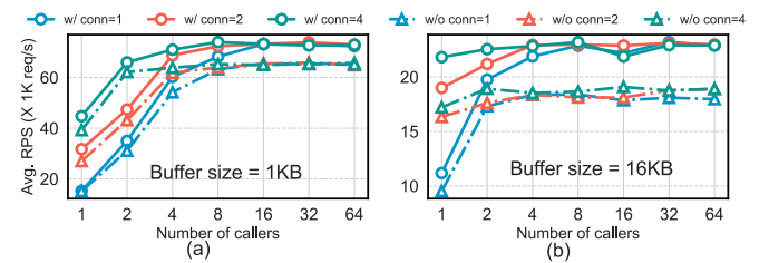
Fig. 12. The total RPS when different caller numbers simultaneously forward data packets of different lengths to a callee. "w/" indicates the introduction of a message queue, and "w/o" indicates no. "conn" represents the number of connections set by wrk. (a) Buffer size = 1KB. (b) Buffer size = 16KB.
